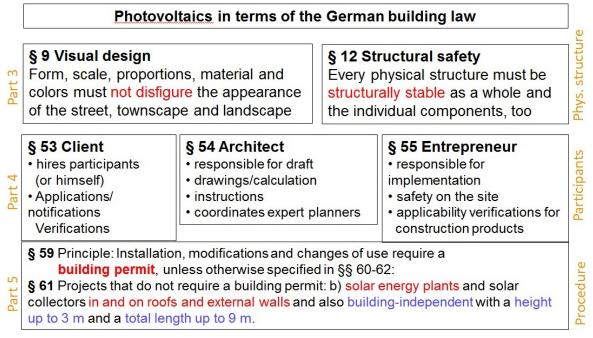
Picture 1 Classification of photovoltaic installations in terms of the building law
