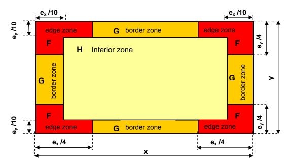
Picture 6 Subdivision of the roof zone areas for ridge roofs and monopitch roofs.
