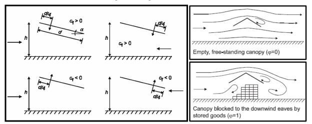
Picture 8 Load assumptions for self-supporting roofs according to EN 1991-1-4
